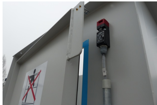
Fig. 83: safety switch inspection door funnel
