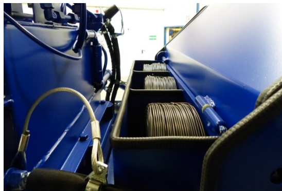
Fig. 77: wire station upper wire
