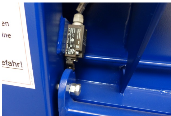
Fig. 11: safety switch, needle flap
