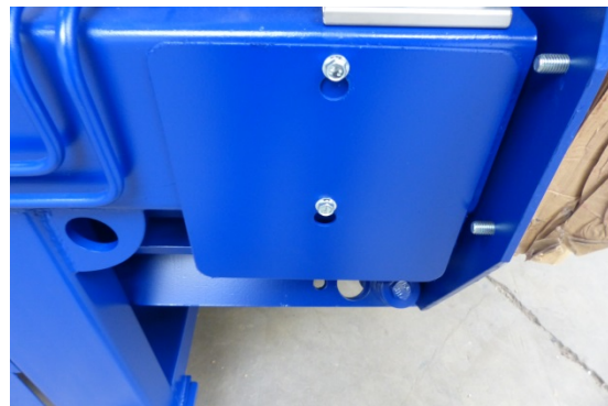
Fig. 4: separating protective devices
