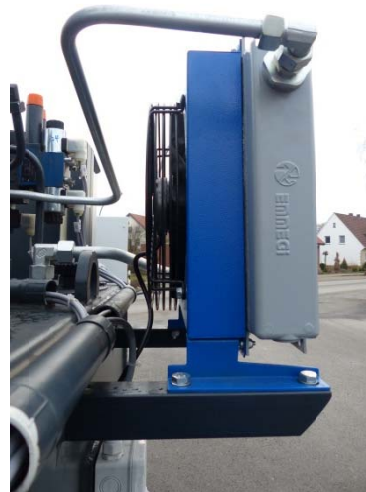
Fig. 87: hydraulic oil cooler/ blower wheel
