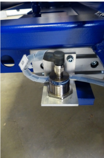
Fig. 57: proximity switch end position needle bottom (right)
