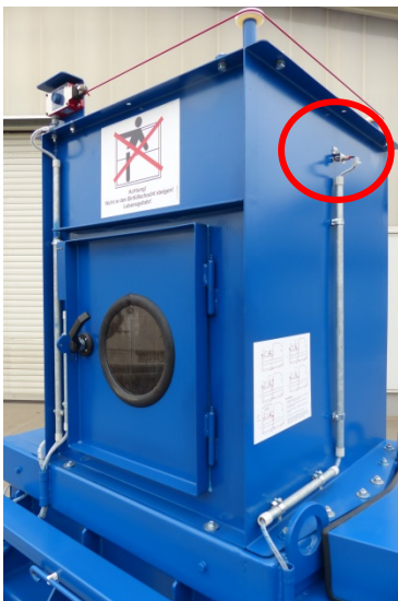
Fig. 63: light barrier level control
