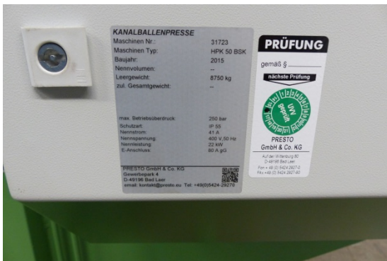
Fig. 2: nameplate & seal of approval for accident prevention
