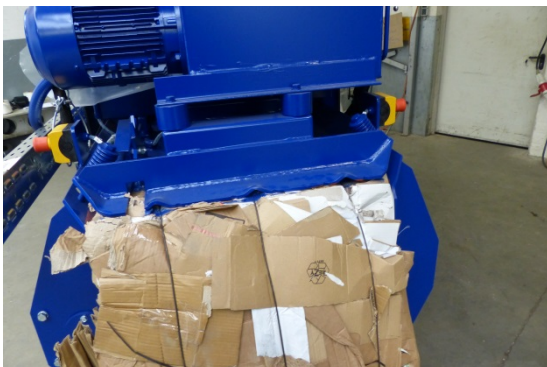
Fig. 51: emergency-stop-button at the end of the press channel
