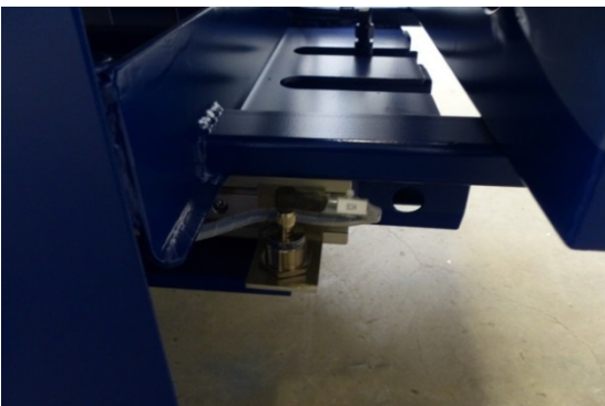
Fig. 58: proximity switch end position needle bottom (left)
