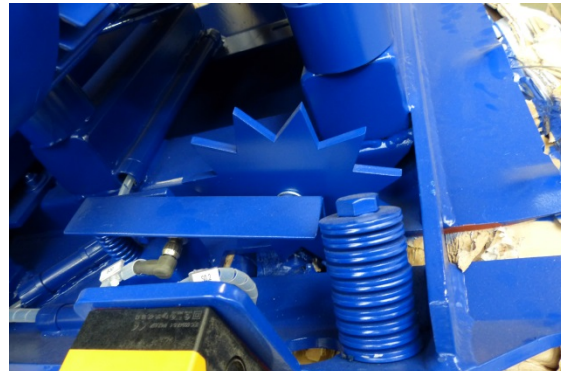
Fig. 61: proximity switch pulse generator bale length
