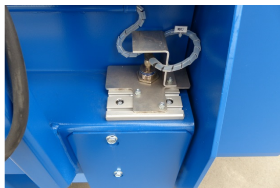
Fig. 55: proximity switch end position press (in front)
