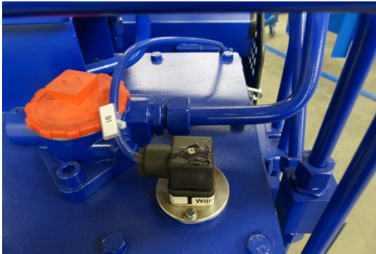
Fig. 62: signaller oil temperature/lack of oil
