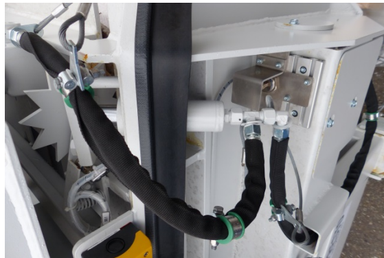
Fig. 86: hydraulic hose with hose protection / detachment protection
