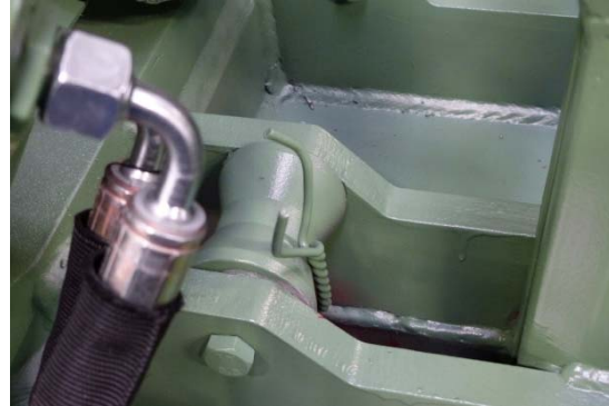
Fig. 32: twisted wire = knot
