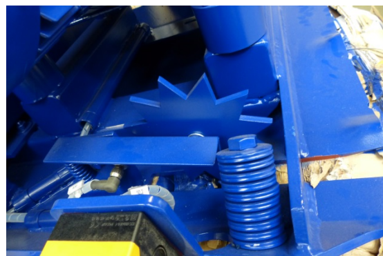
Fig. 29: bale length measuring wheel
