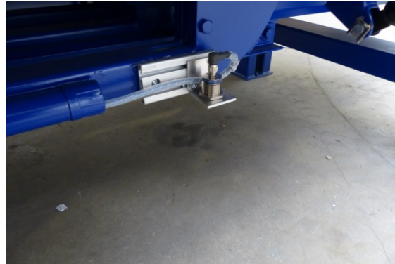
Fig. 59: proximity switch end position needle at top (right)
