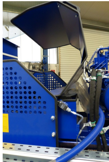
Fig. 12: safety switch, knotting hood
